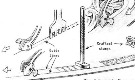
The Adjustable Creaser is also good for making guide line for rope & geometric stamping.
