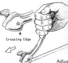
Adjust the Creaser to desired width and push firmly along the edge. Hold as shown, not quite so straight up as with the single line creaser. You can also move it back and forth.
